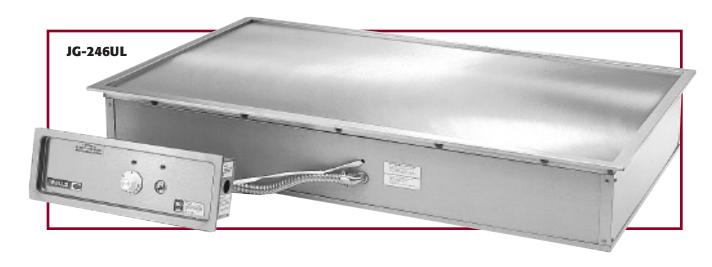
Wells JG-246UL Built-In Griddle is essential for any kitchen preparing "Teppan" style dishes. The recessed griddle plate has a 20" x 24" high temperature (up to 550°F) cooking area that is ideal for stir-frying.
