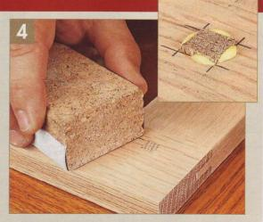
▲ Finish up by gluing a 3/8" x 3/8" peg into the mortise. Leave the peg slightly proud, and then sand it flush with the surface after the glue dries.
