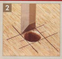
Next, use a chisel, and cut across the grain to establish the first edge of the mortise. By cutting across the grain first, you will prevent the the wood from splitting during the next few cuts.
